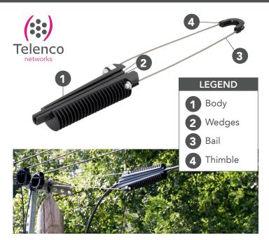
The ACADSS C clamps are designed for the anchoring of FTTH aerial round cables from 6mm up to 14mm, with reinforced outer sheath. They are used on poles or facades, with maximum spans of 90m.
